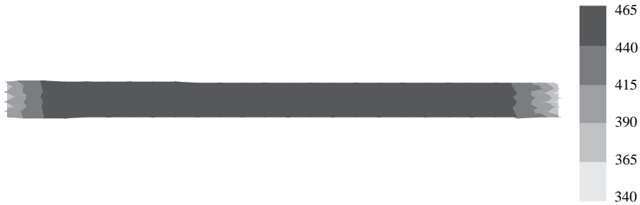
Figure 3.10: Calculated tensile stress distribution in the sample at 15 % of tensile strain.
